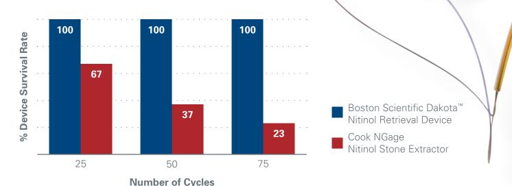
In a Bench Study, Dakota's Retrieval Device demonstrated to be more durable than the NGage Stone Extractor when capturing larger stones ranging from 8mm – 10mm. 100% of the Dakota Retrieval Device survived 75 cycles without breakage compared to 23% of the NGage retrieval device.<sup>1</sup>
