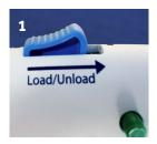
Push the green load button to expose the red portion of the toggle button.
